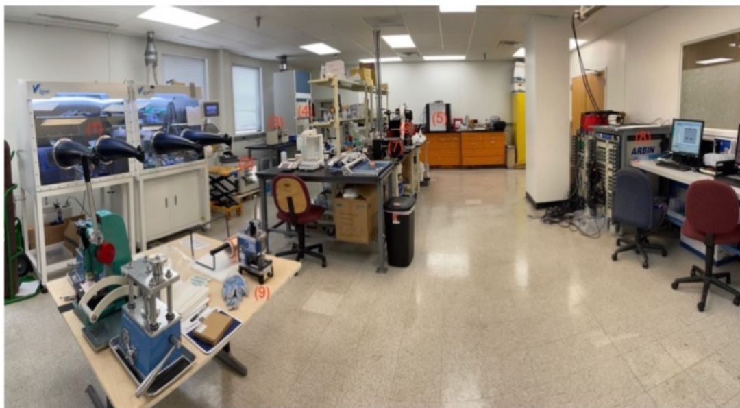
Inside of WHP's lab facility, showing (1) glovebox and pouch cell sealer, (2) vacuum oven, (3) heated calendaring, (4) fume hood, (5) constant temperature storage for battery testing, (6) pouch cell electrode stacker, (7) ultrasound welder, (8) Arbin doctor's blade coater, Landt battery testers electrode die cutter, pouch former.
